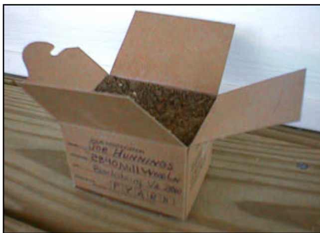
Figure 11. A full soil sample box properly labeled with name, address, and sample identification.
