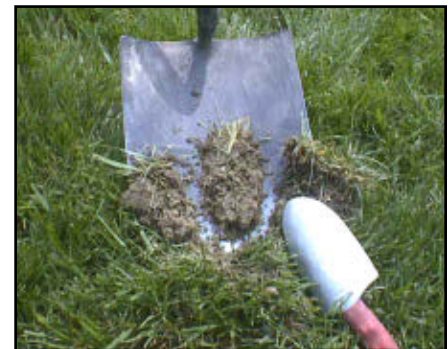
Figure 8. An example of creating a ribbon of soil from the initial slice.
